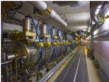
Fig. 7.26 Principle of the acceleration of charged particles in a cylindrical resonating cavity. The resonator is excited in the "TM 010 mode", in which the electric field is oriented parallel to the z axis, and the magnetic field in azimuthal direction.
