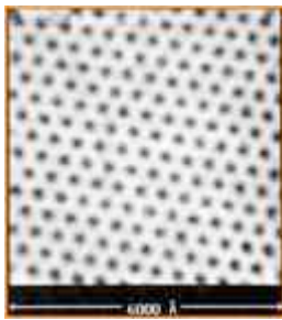
Scanning Tunneling Microscopy NbSe2, 1T, 1.8K
