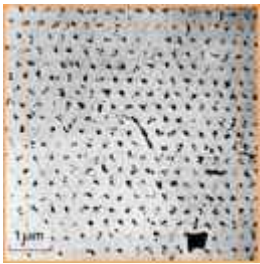
U. Essmann and H. Trauble Max-Planck Institute, Stuttgart Physics Letters 24A, 526 (1967) Bitter Decoration Pb-4at%In rod, 1.1K, 195G
