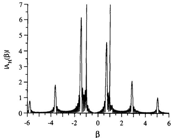
Fig. 7. Modulus of the angular spectrum of the field diffracted at 5 GHz by an array of 20 cylinders with 3 mm radius ( $ka=0.3$ ), spaced by 28 mm ( $kd=2.9$ ) and evaluated on a plane at 3.5 mm ( $kh=0.35$ ) from their axes. The grating is illuminated by a plane wave at a  $45^\circ$  incidence angle.
