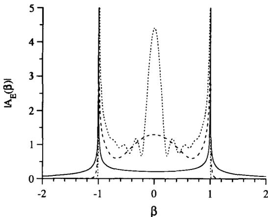
Fig. 6. Modulus of the angular spectrum of the field diffracted by a single cylinder for three different radii:  $ka=0.15$  (full line),  $ka=3.14$  (dashed line) and  $ka=12.56$  (dotted line) evaluated at a distance  $ky=1.5ka$ .
