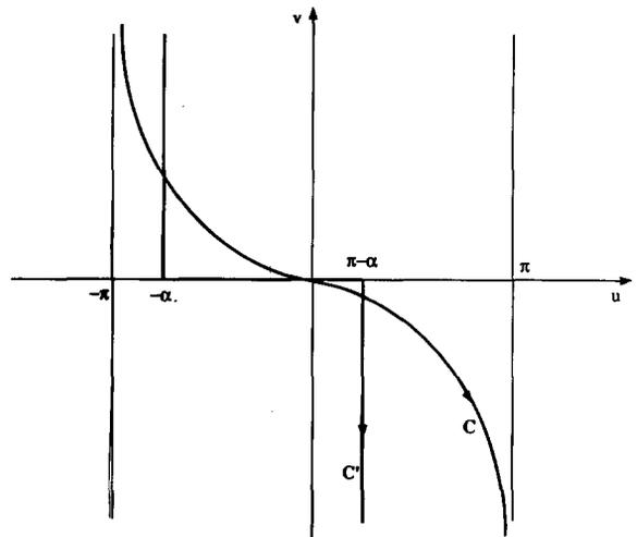
Fig. 2. Two possible integration paths for the evaluation of the function  $H_n(\rho)$  in eq. (2).
