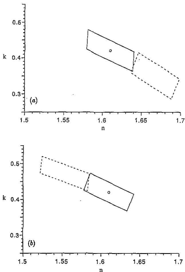
Figure 3. Error parallelograms centred on the right (full line) and wrong (broken line) solutions for the optical constants  $n$  and  $k$ , in correspondence to (a)  $\gamma = 3.03$  and (b)  $\gamma = 3.24$ . The true values of the optical constants are  $n = 1.61$  and  $k = 0.42$ ; the real refractive index of the coating film is  $n_2 = 1.95$ . The per cent errors in the reflectivities  $R_1$  and  $R_2$  amount to 4%.
