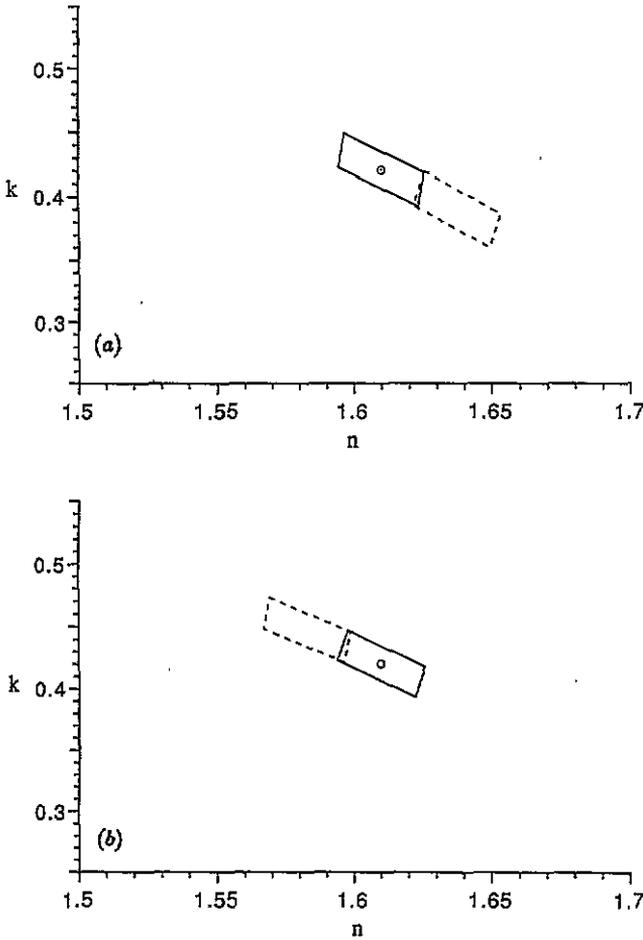
**Figure 2.** Error parallelograms centred on the right (full line) and wrong (broken line) solutions for the optical constants  $n$  and  $k$ , in correspondence to (a)  $\gamma = 3.09$  and (b)  $\gamma = 3.19$ . The true values of the optical constants are  $n = 1.61$  and  $k = 0.42$ ; the real refractive index of the coating film is  $n_2 = 1.95$ . The percent errors in the reflectivities  $R_1$  and  $R_2$  amount to 2%.
