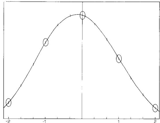
Fig. 4. Theoretical (full line) and experimental (heavy dots) intensity distribution in the image of two unresolved point sources. Encircled experimental points have been used for the correction procedure. Nyquist distance is taken as unit on the  $x$ -axis.
