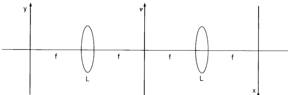
Fig. 1. Image forming system considered for describing the postprocessing method. L represents a converging lens of focal length  $f$  and the  $y$ -,  $\nu$ - and  $x$ -planes represent the input (object), pupil and output (image) planes, respectively.
