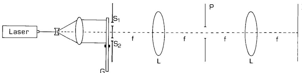
Fig. 3. Experimental setup used for testing the superresolving method. G: rotating ground glass;  $S_1, S_2$ : secondary spatially incoherent sources; L: converging lens of focal length  $f$ ; P: low-pass filter; I: image plane.
