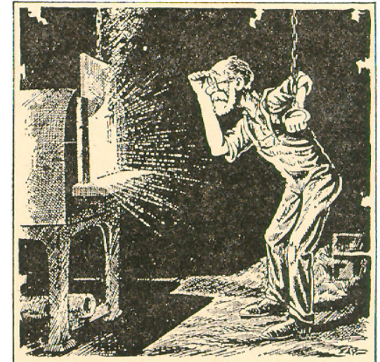
The first optical pyrometer (from Heat and Temperature Measurement , by R. L Weber, 1950)
