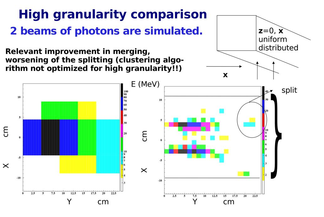
At the beginning, no improvement was observed in merging reason: the algorithm merges everything in 20 cm. The KLOE clustering algorithm cannot be easily adapted for high granularity read-out.
