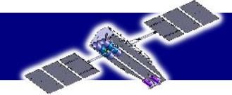
POLARIX: 3 Jet-X optics with 3 GPDs working in 2-10 keV energy range
