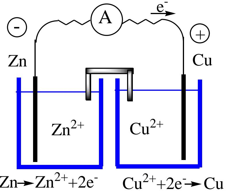
$$E_+ = E_{\text{Cu}^{2+}/\text{Cu}} = E_{\text{Cu}^{2+}/\text{Cu}}^0 + \frac{0,0592}{2} \log [\text{Cu}^{2+}]$$
