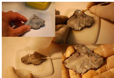
Cleaning a siderite with Nitol solution to obtain the Widmanstätten pattern.
