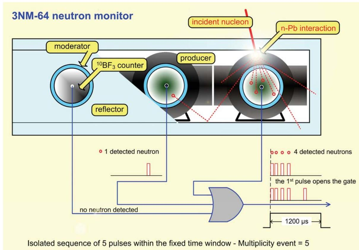
*The figure illustrates the production of multiplicity events in a 3NM-64 providing a sketch of a multiplicity 5 event detection.*
