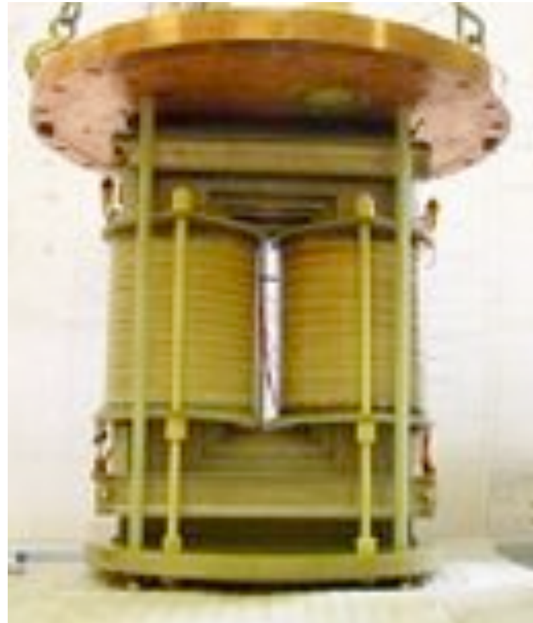
41 kVA superconducting transformer European project READY
